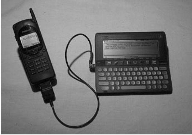
Figure 6.8 A GSM phone connected to a palmtop.
